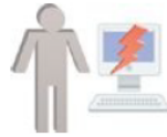
Figure 2.7. The notation used for an attack originating from a workstation. The human symbol is optional.
